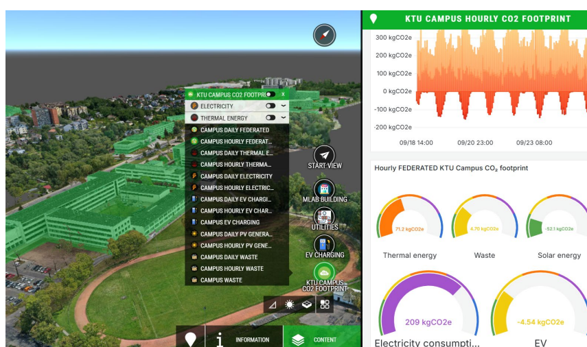
Kaunas University of Technology campus digital twin model for operational carbon footprint assessment
